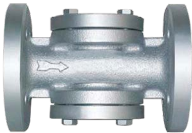
SG-40 Sight Glass Flanged Ends Flanged Ends : JIS-10K/ANSI-150LB, DIN3202 PN16-F1 Material : Cast Iron / CF8 /CF8M Size : 1/2" ~ 8"
