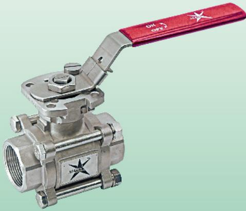
Mars V-Control Ball valves match the control performance of globe valve, excellent for modulating service, but Mars V-Control ball valves are more compact, lighter weight, and much less expensive than globe valves.
